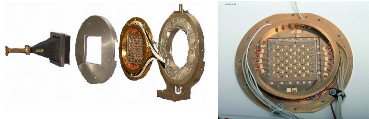
Figs. 2a, b and c A 25 W, Ka band spatial amplifier array with hard horn feed
